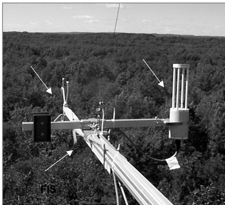
Figure 2.3: Isoprene flux instrumentation mounted on the UMBS~Flux tower.
