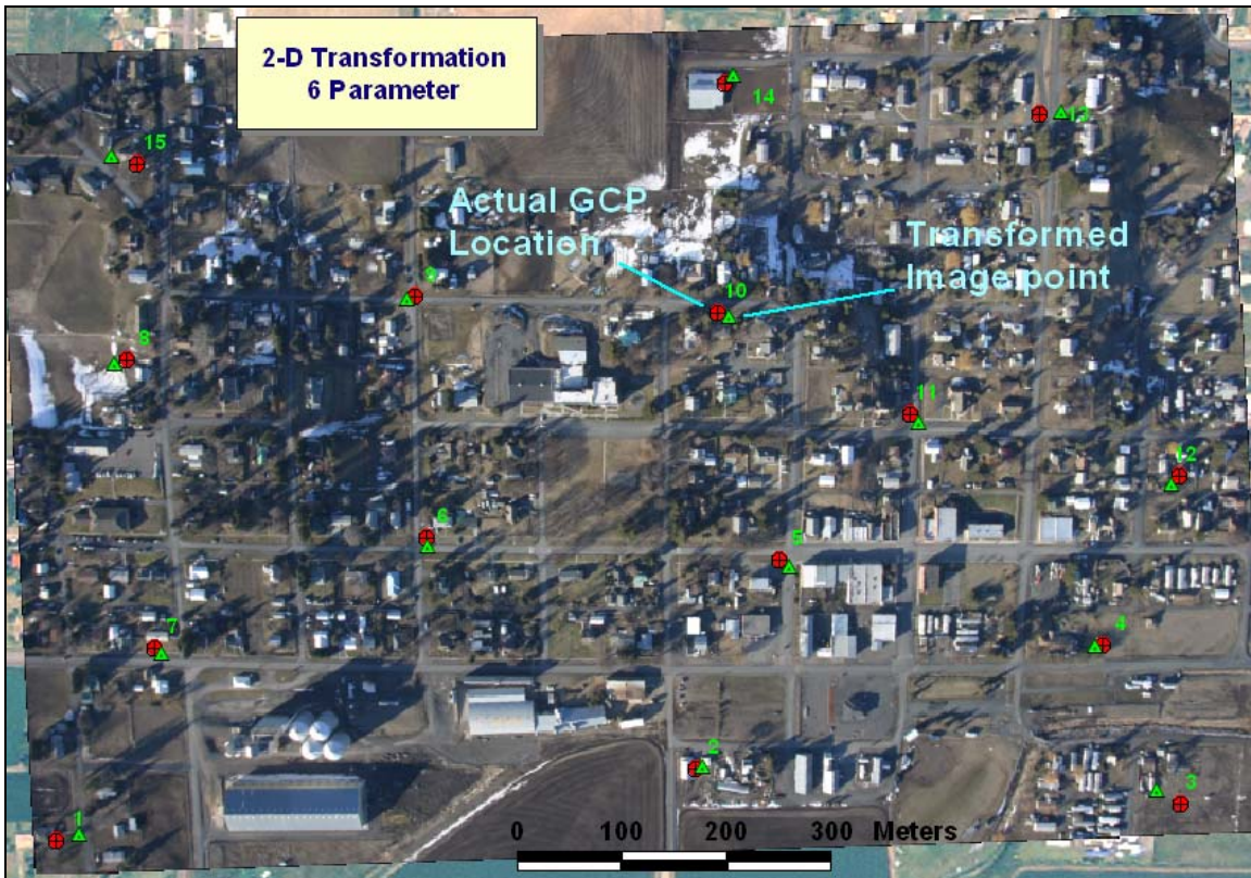
Figure 3.47 Aerial image georeferenced with 6 parameter 2D transformation.
