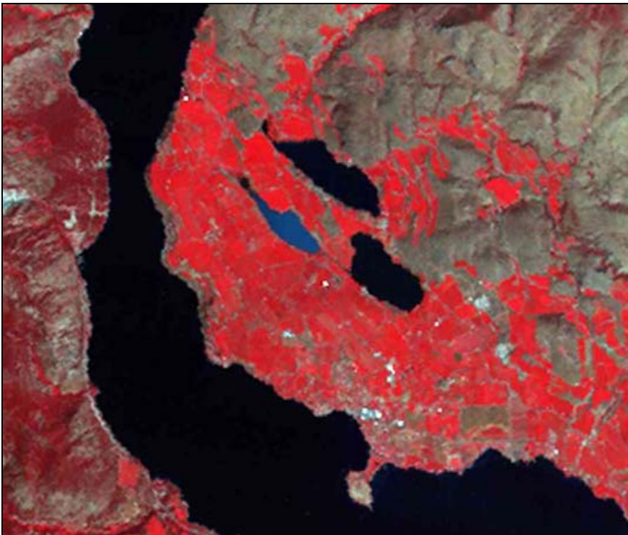
Figure 5.12 Chlorophyll reflectance in a Landsat 5 visible-near infrared image of Manson Lakes, July 23, 1988
