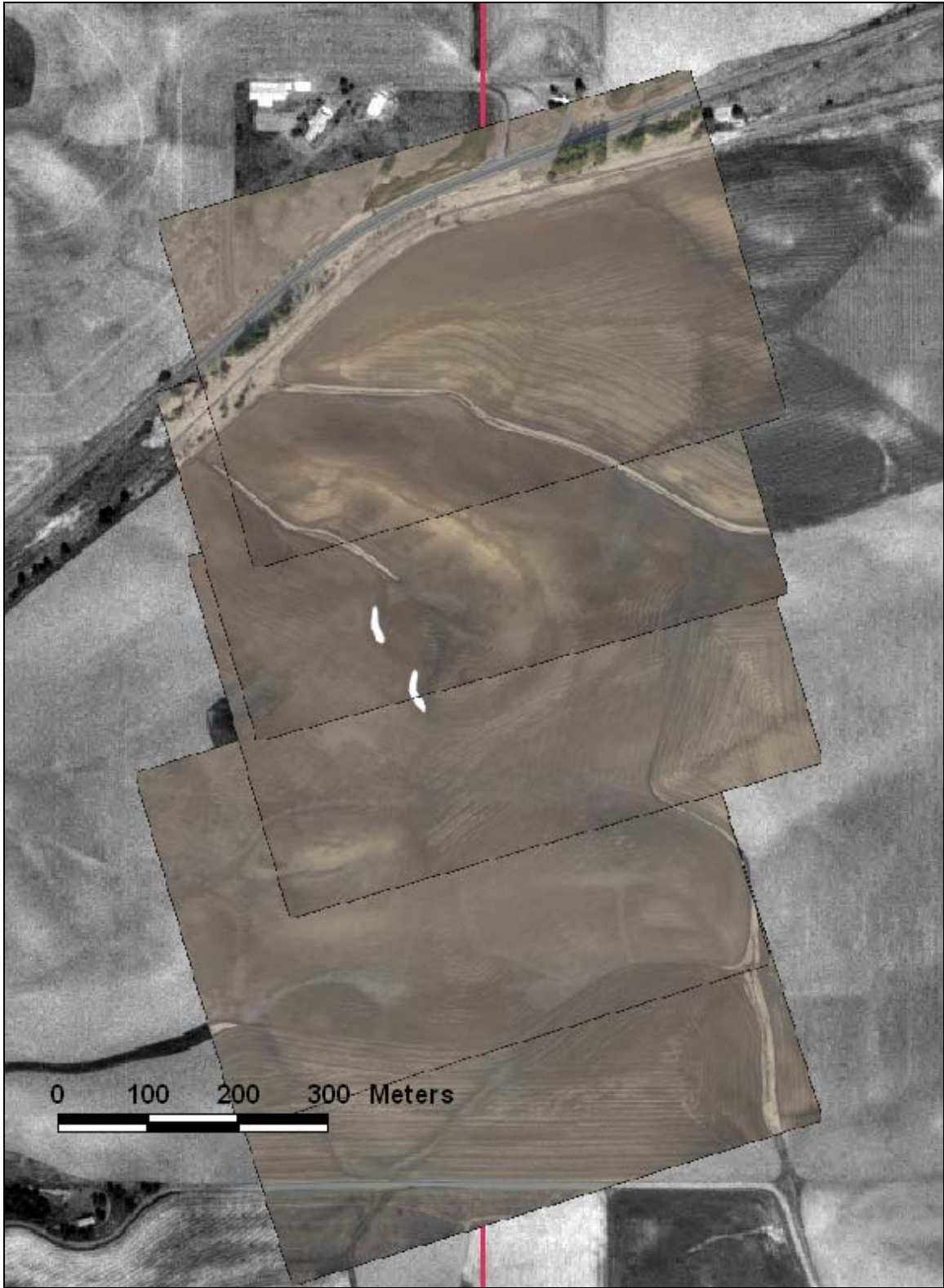
Figure 3.40 Completed sequence of georeferenced aerial images.
