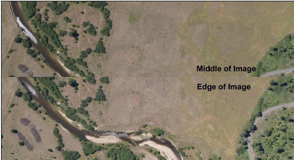
Figure 3.12 Image falloff detection in high-resolution digital aerial images.
