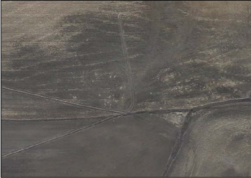
Figure 8.22 Constructed field drainage channels, March 15, 2004.
