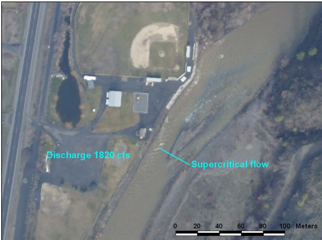
Figure 6.51 Supercritical flow and hydraulic jump in the January 31, 2004 aerial image.
