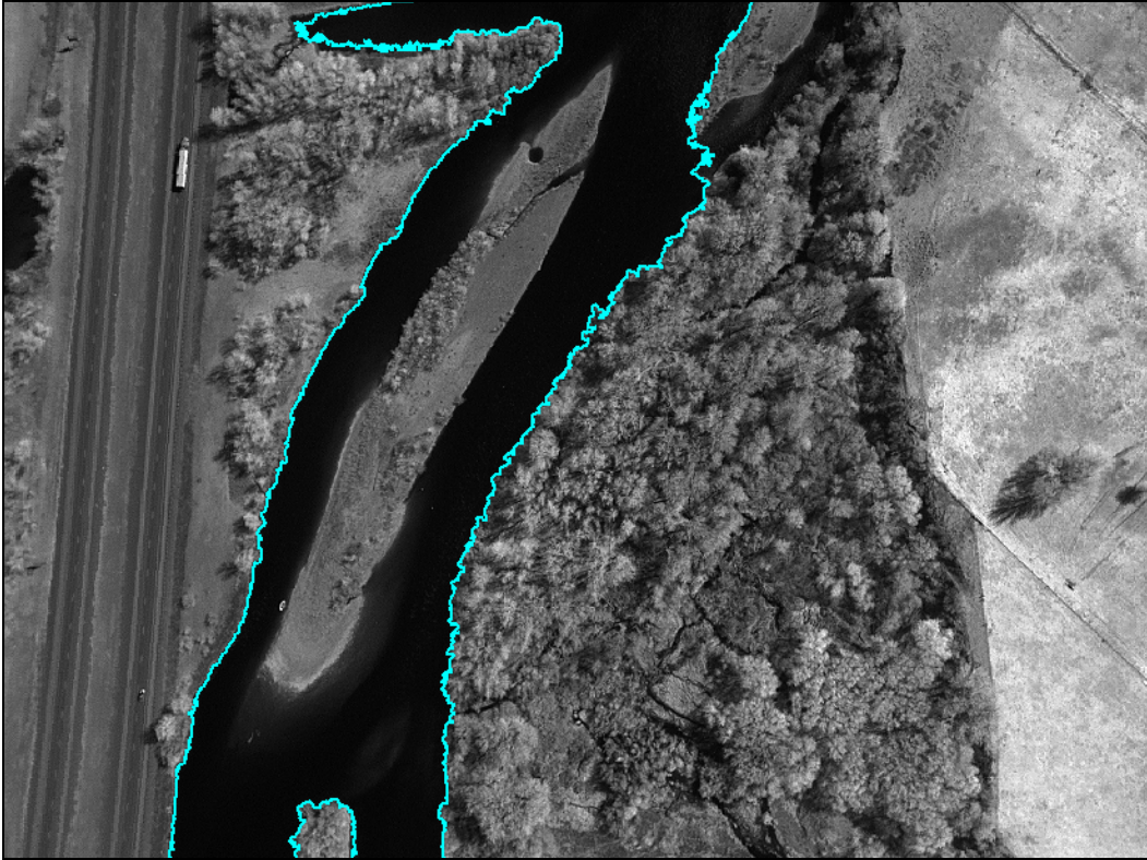
Figure 6.13 Automatic extraction of water surface boundary (light blue) from a single band infrared image.
