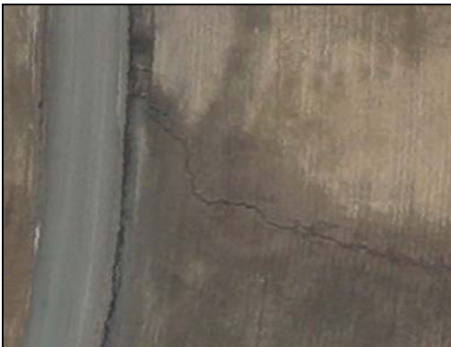
Figure 8.16 Termination of a multi-thread ephemeral gully in a permanent drainage channel (road ditch).
