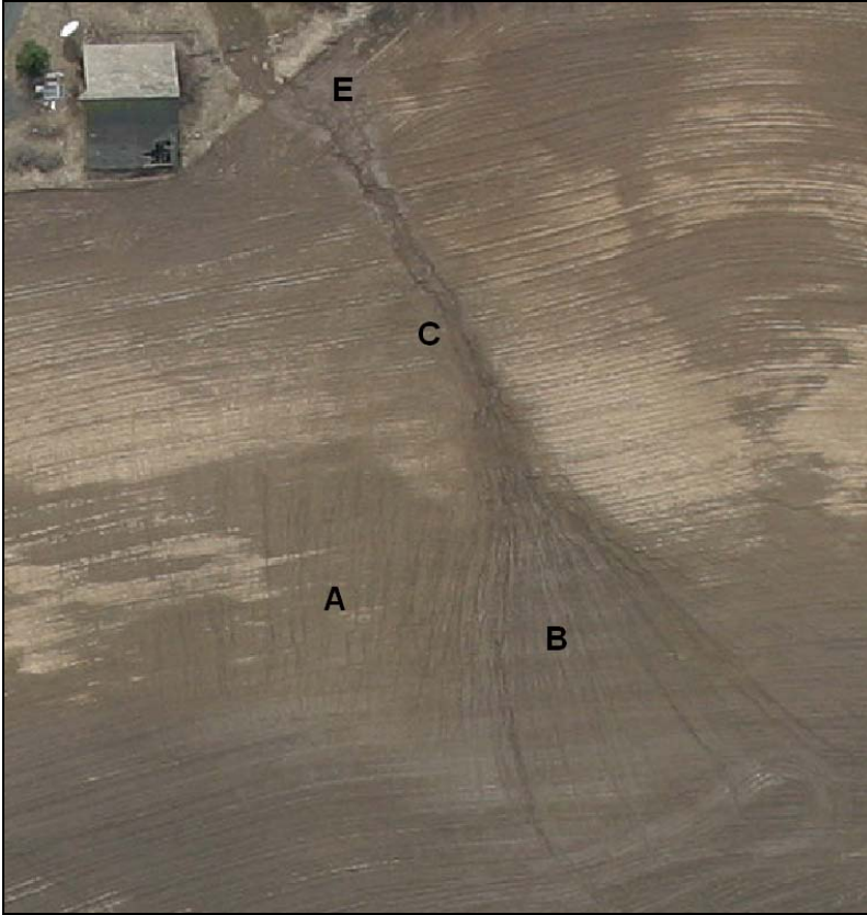
Figure 7.4 Natural color vertical aerial image of an ephemeral gully system, March 13, 2004.
