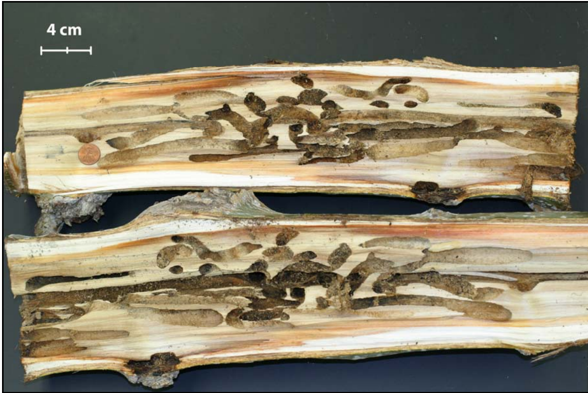
Figure 4. Photograph of split log showing heavy damage from Prionoxystus robiniae (Peck) larvae galleries. For a reference size, note the penny on the left hand side of the upper log.
