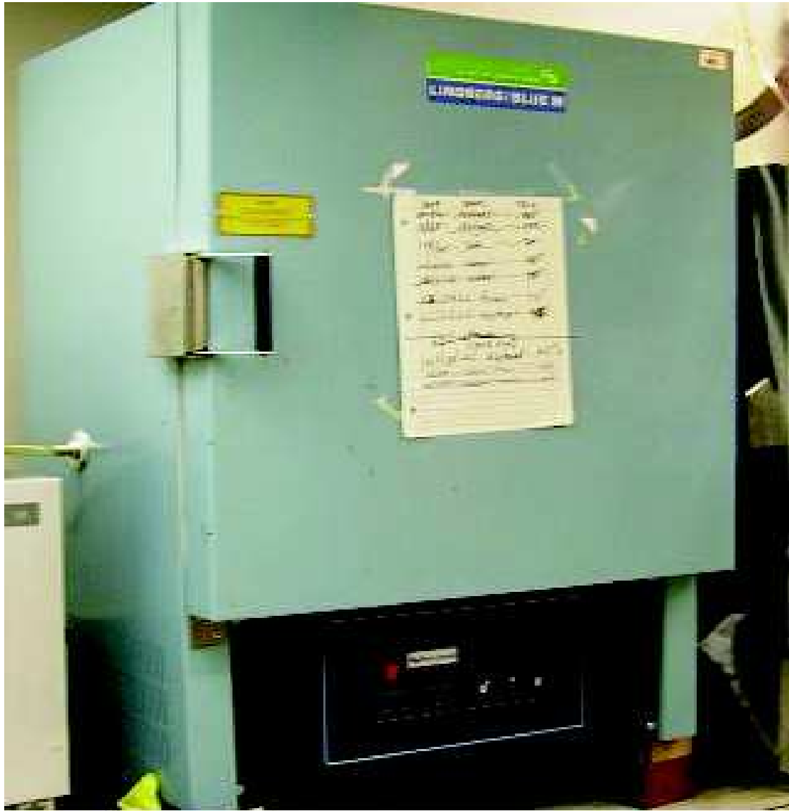
Figure 3.3: Oven used to polymerize sample.
