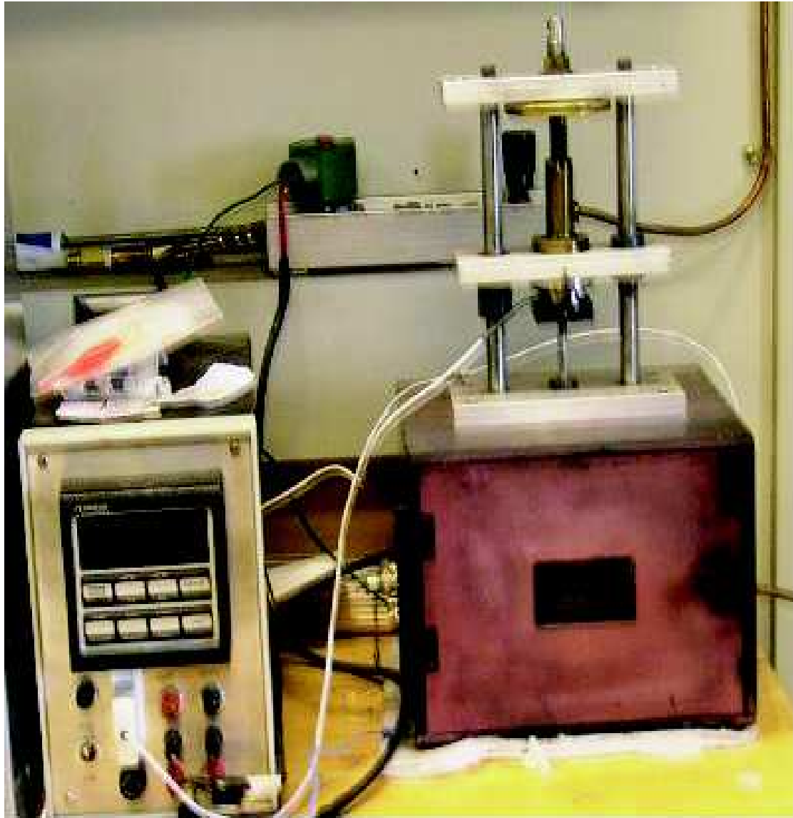
Figure 3.4: Oven (right) used to press samples. The mechanism above the oven is used to apply pressure and the unit to the left is the temperature controller.
