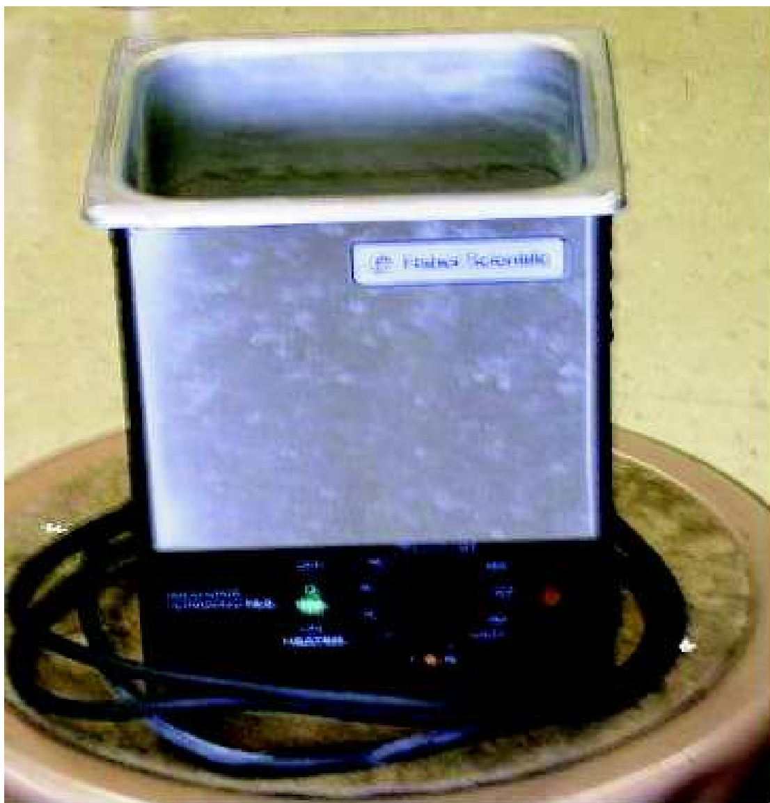
Figure 3.1: The Ultra-Sonic bath used for dissolving DO11 in MMA. The heating system of the bath is turned off to avoid polymerization. Polymerization in the ultra-sonic bath yields solution that are difficult to filter and eventually to bad sample quality.
