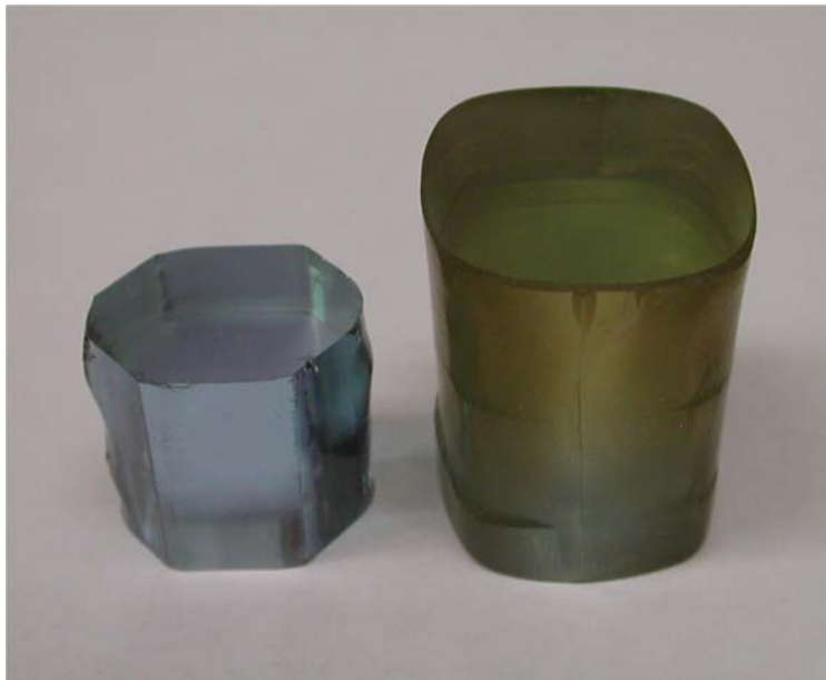
Figure 3.2: Photograph of a hexagonal a -axis (left) and a rectangular c -axis (right) grown \text{Nd:YVO}_4 boules.
