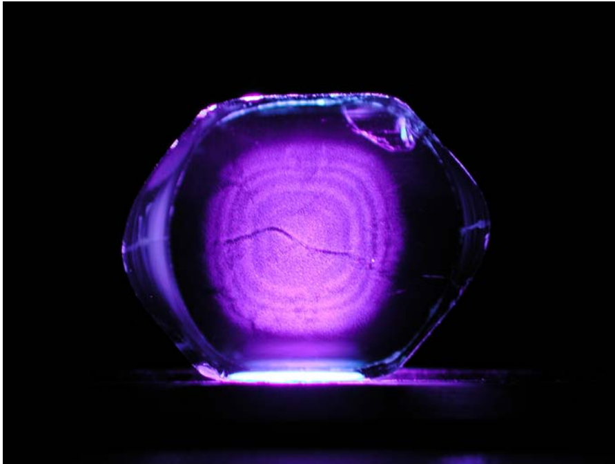
Figure 3.18: Photograph of small “growth ring” void clusters in a Nd:YVO 4 boule using UV illumination.
