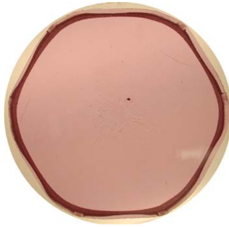
Figure 2.8: Slice of Nd:YAG boule showing hexagonal structure from faceting during growth. The boule slice is 75mm from top to bottom of the photograph.
