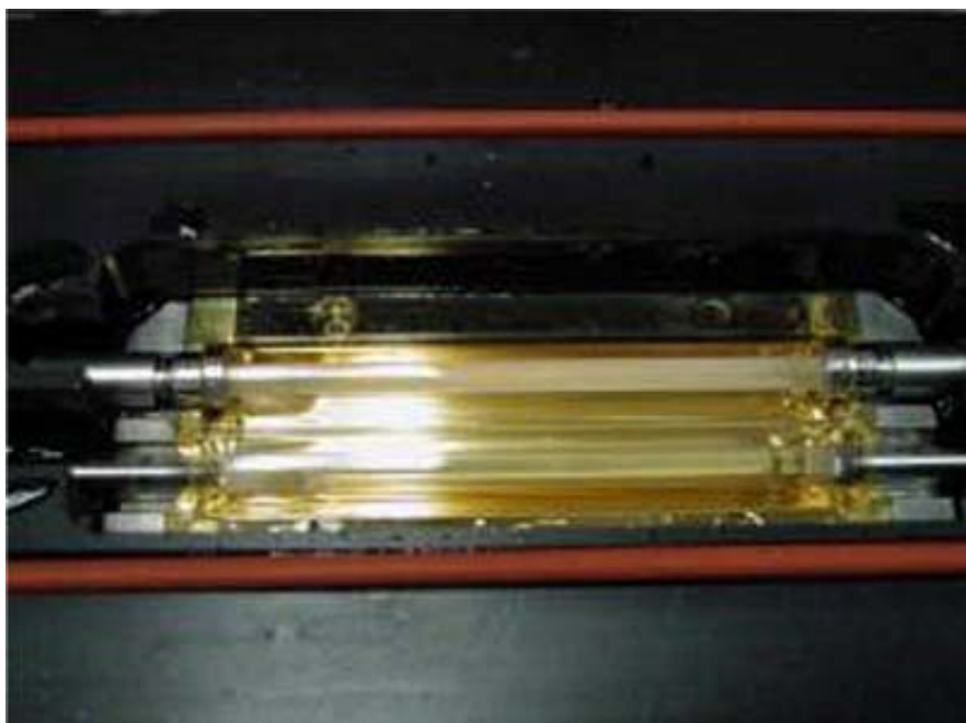
Figure 6.1: Photograph of inside of Control 512 laser cavity. The rod on the top is the Nd:YAG rod and is 79mm in length, and the rod on the bottom is the krypton-arc lamp.
