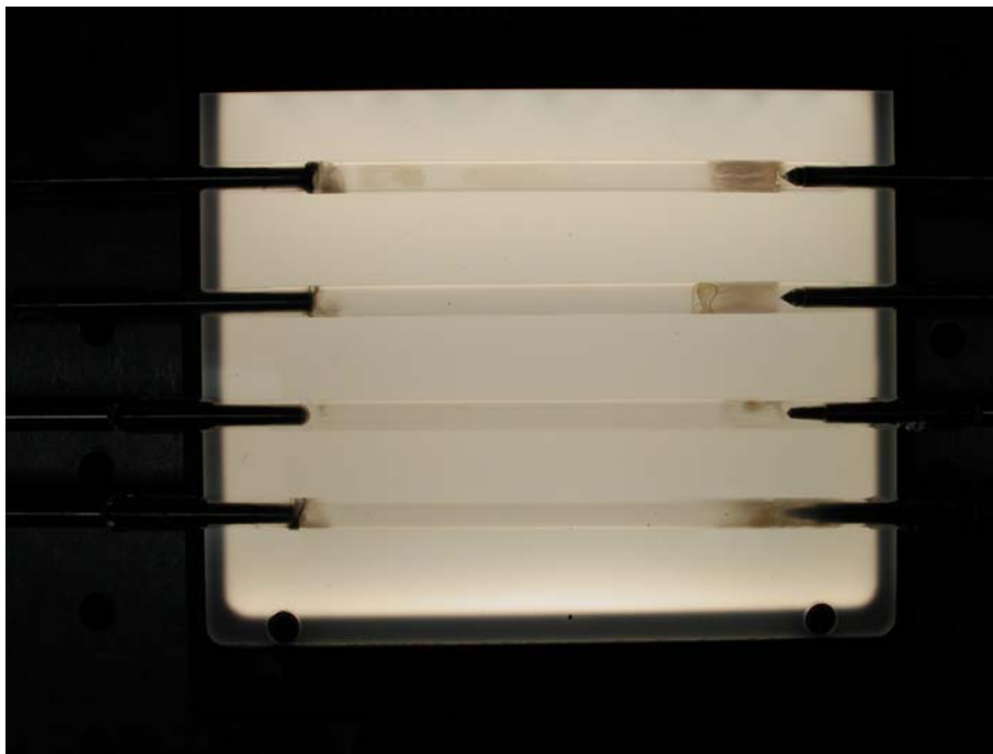
Figure 6.11: Wall darkening in krypton-filled arc lamps seen after several uses.
