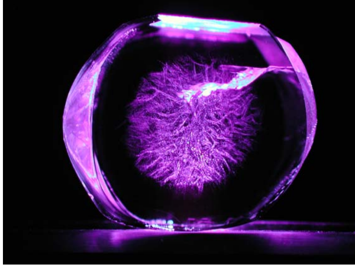
Figure 3.20: Photograph of small “brain coral” void clusters in a Nd:YVO 4 boule using UV illumination.
