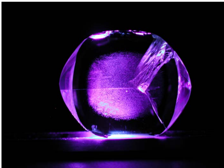
Figure 3.19: Photograph of small void clusters in a Nd:YVO 4 boule using UV illumination.
