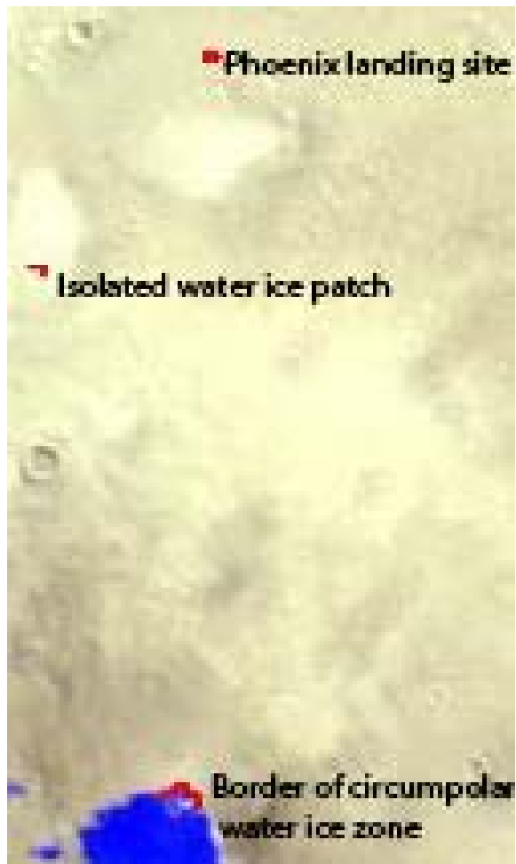
Fig. 4-12 The occurrence of surface water-ice in OMEGA image orb1034_3. Marked in red are the Phoenix Landing Site or the borders of surface water-ice occurrences.
