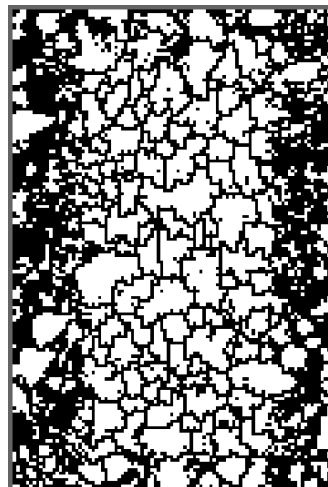
Figure B.43 Results of Canny Operation (a) Mastic Phase, (b) Aggregate Phase; Results of Watershed Image Segmentation (c) Mastic Phase, (d) Aggregate Phase; SL Superpave-C
