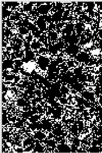
Figure B.37 Results of Canny Operation (a) Mastic Phase, (b) Aggregate Phase; Results of Watershed Image Segmentation (c) Mastic Phase, (d) Aggregate Phase; SL CMHB-C
