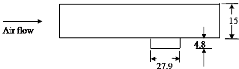
Figure 5.2. A cross-section view of the convective emission chamber test-section (all dimensions in cm but not to scale)
