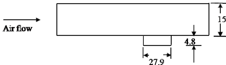
Figure 4.3. A cross-section view of the convective emission chamber test-section (all dimensions in cm but not to scale)
