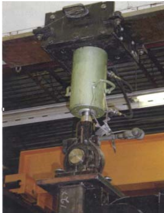
Figure 3.31 Axial Load Trolley System
