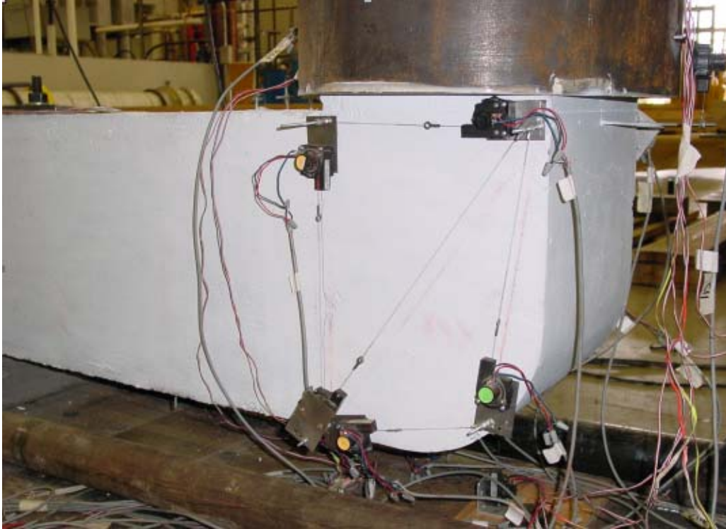
Figure 3.32 View of Joint Panel Instrumentation
