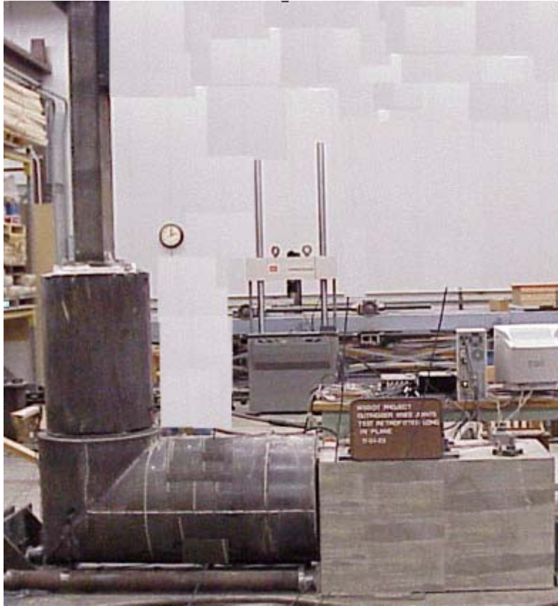
Figure 3.16 Overall View of the Retrofitted Long Outrigger Specimen
