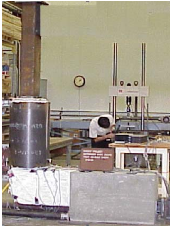
Figure 3.12 Overall View of the As-Built Short Outrigger Specimen
