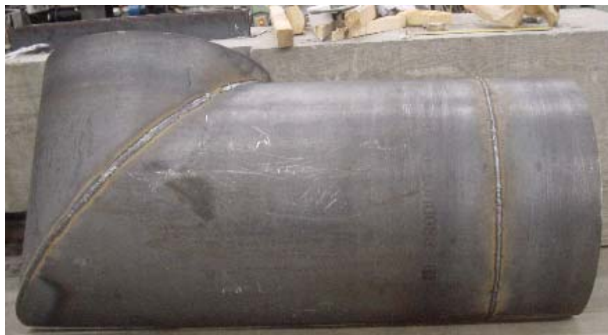
Figure 6.18 A Picture of the Clamshell Used in the Retrofit of the Beam-Joint
