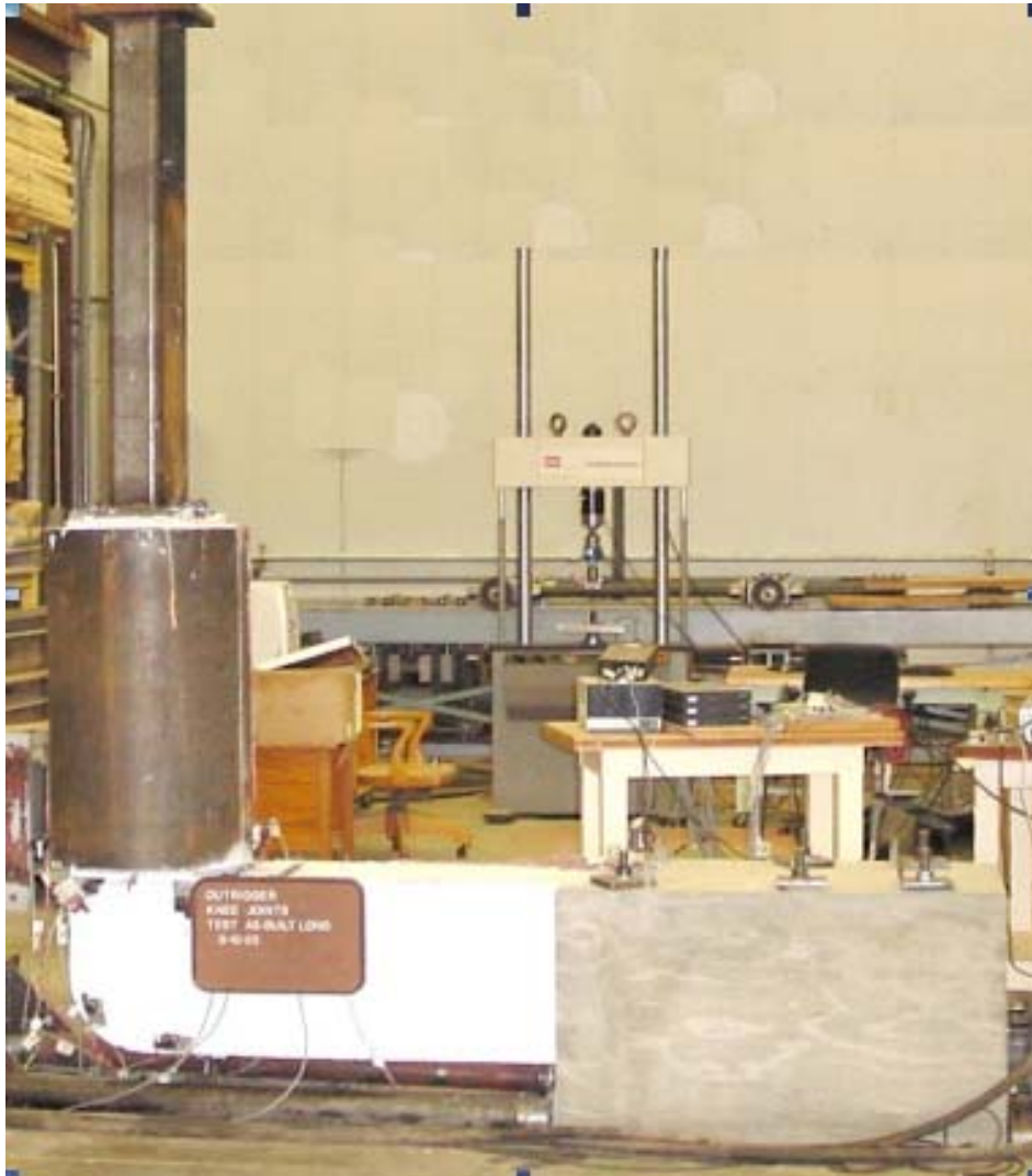
Figure 3.8 Overall View of the As-Built Long Outrigger Specimen
