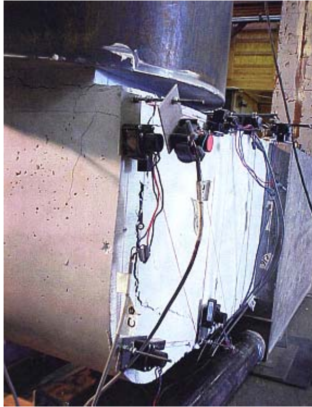
Figure 4.13 Bond Splitting Cracks on the Back Face of Specimen ASI
