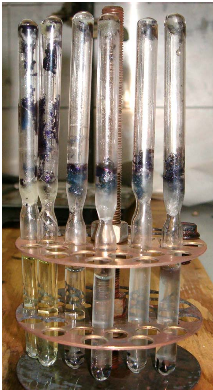
An example of experimental sulfide synthesis samples after the experimental run. Width of tubes is 1cm.
