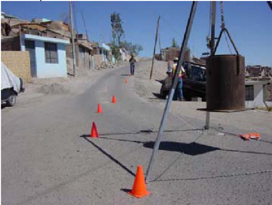
Figure A.41 Photograph of SASW testing at site of Calle Nueva
