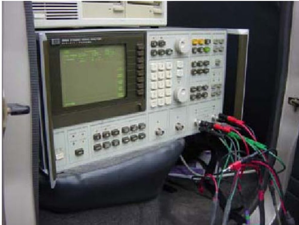
Figure 3.3 HP 3562A dynamic signal analyzer.
