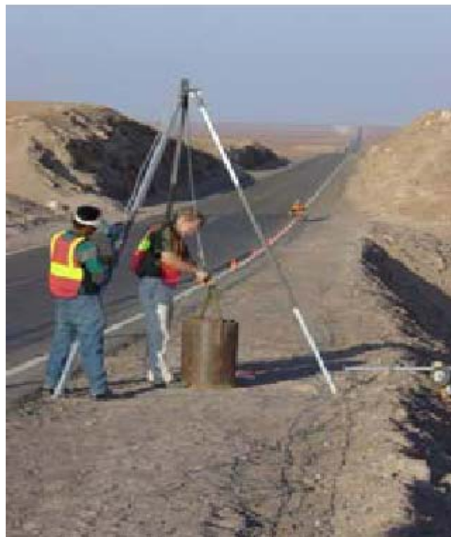
Figure A.60 Photograph of SASW testing at site of Valley Fill
