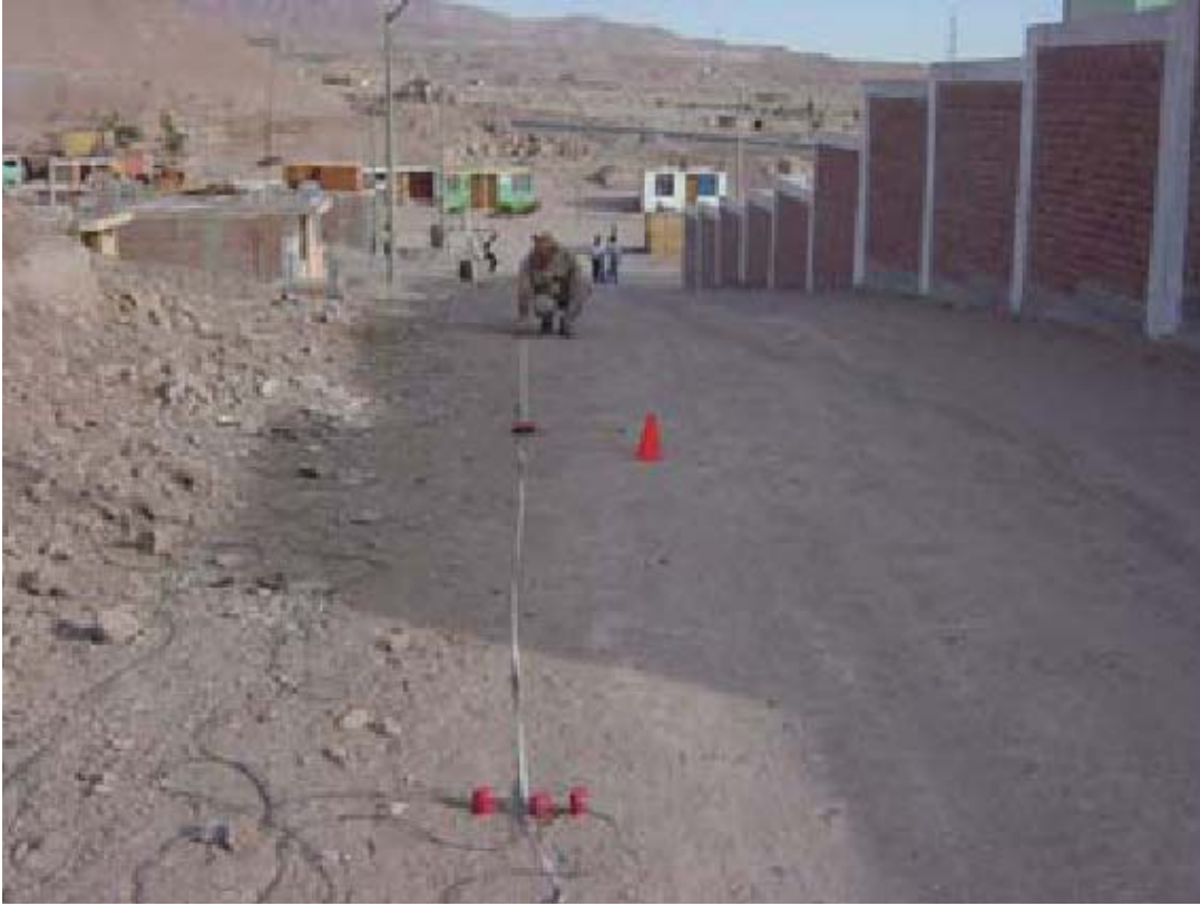
Figure A.50 Photograph of SASW testing at site of San Antonio Hospital 700
