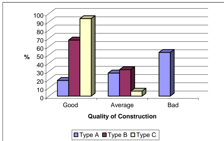
Figure 5.1 Damage distribution by quality of construction (Fernandez et al. 2001).
