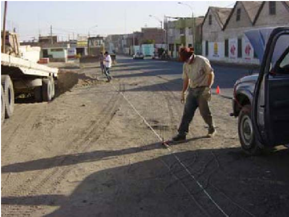
Figure A.38 Photograph of SASW testing at site of Colegio “Coronel Bolognesi”
