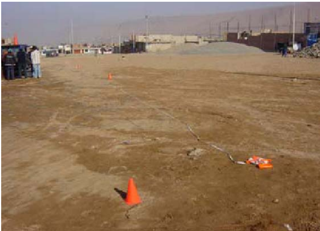
Figure A.25 Photograph of SASW testing at site of Municipal Gas Station
