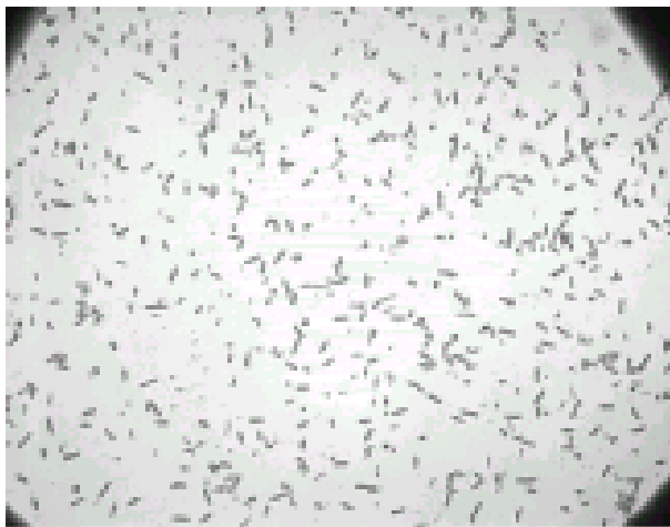
Figure 4.3.1G: AMC Microscope image of NCO-coated silicon wafer (control) after exposure to E. coli -TSB solution 29 hours.
