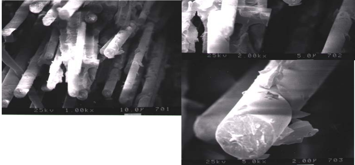
Figure 6.3.4.3C: Scanning electron microscopy (SEM) of Greige Fiber tensile fracture.
