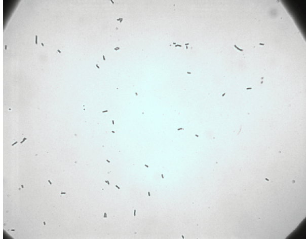
Figure 4.3.1F: AMC Microscope image of Tetracycline coated silicon wafer after exposure to E. coli -TSB solution 29 hours.
