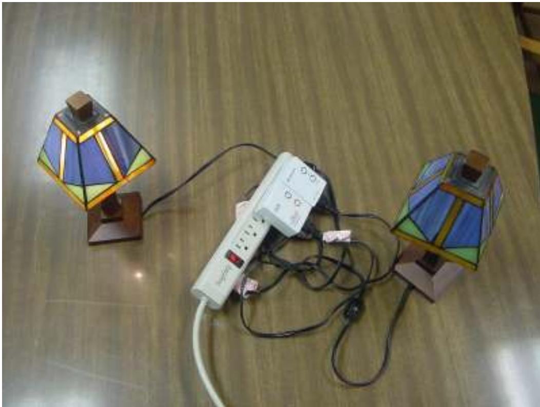
Figure 3. X-10 Lamp module [8].
