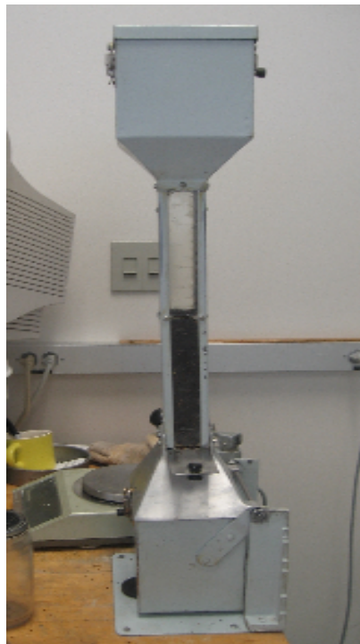
Figure 1- Apparatus for measuring volume by rapeseed displacement
