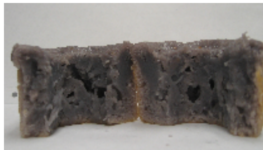
Figure 7- Transversal cut of RM
