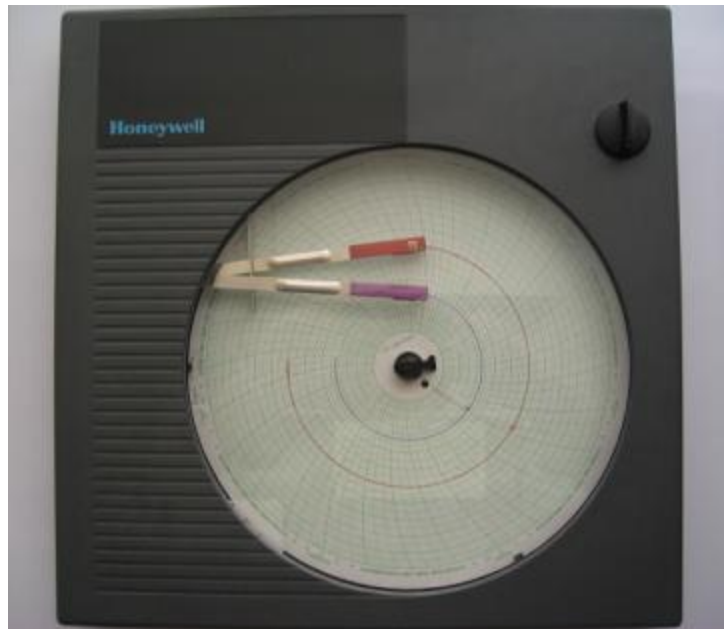
Figure 3.2: Honeywell chart recorder with the red pin recording the humidity and the blue pin recording the temperature.
