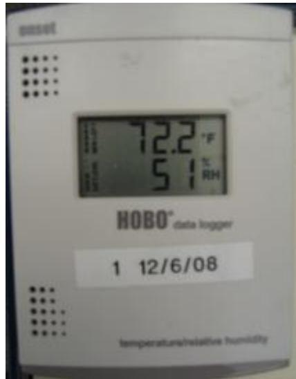
Figure 3.3: Hobo data logger showing the temperature (°F) and relative humidity.
