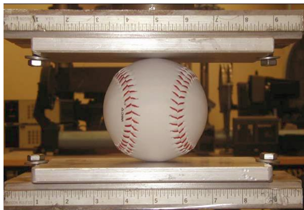
Figure 2.3: Testing apparatus to measure ball compression
