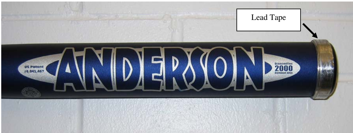
Figure 3.17 - Method of Increasing MOI of Weight Group
