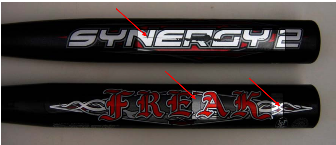
Figure 3.12 - Visible Damage Resulting from BCT Treatment
