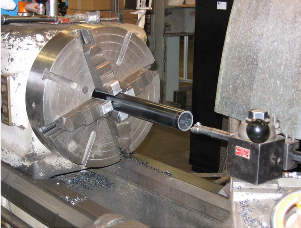
Figure 2.15 - Setup for boring down the inside diameter of a bat
