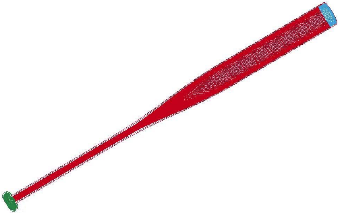
Figure 5.10 – Sectioned view of single wall aluminum bat model
