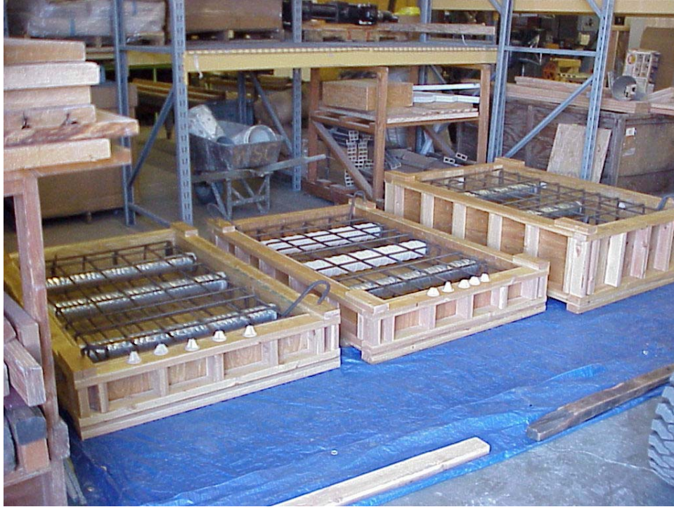
Figure 3.1 - Formwork, rebar and post-tensioning ducts in 20 cm (8 in) and 40 cm (16 in) thick specimens (Pearson, 2003)
