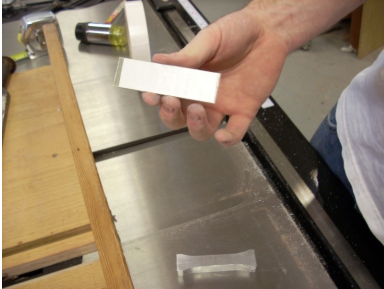
Fig 4.4-14: Double Sided Tape Applied to Prepared Composite Strip
