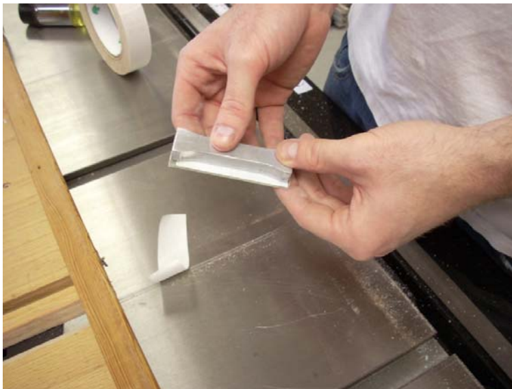
Fig 4.4-15: Aluminum Template Taped to a Prepared Composite Strip
