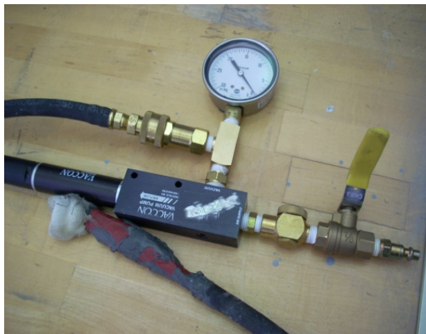
Fig 4.2-8: Vacuum Pump Used for VIM Lay-Up
