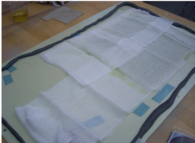
Fig 4.2-11: Cheesecloth Setup for the VI Process
