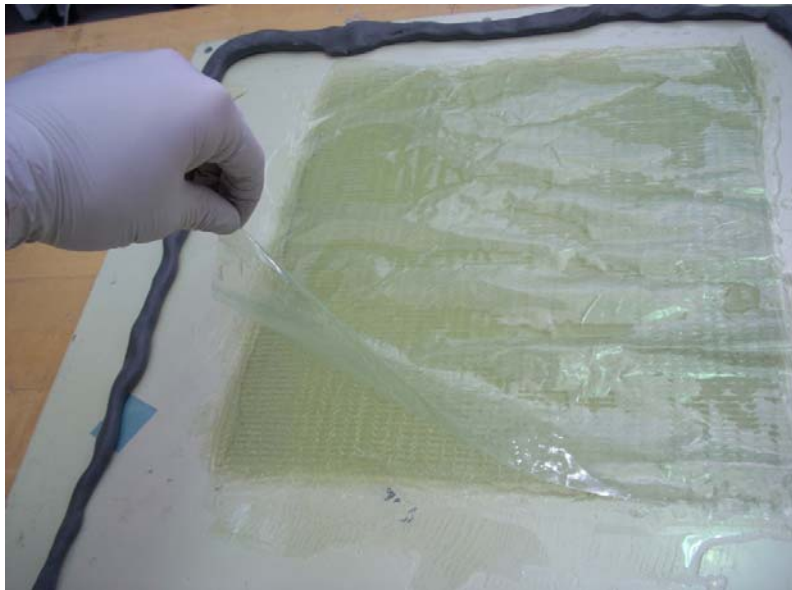
Fig 4.2-10: Top Anti-Bond Seal Being Placed Over Prepared Infusion Laminate
