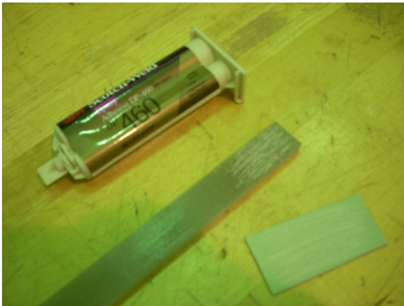
Fig 4.4-10: Materials Prepared for Tab Adhesion (Epoxy, Specimen, & Tab)
