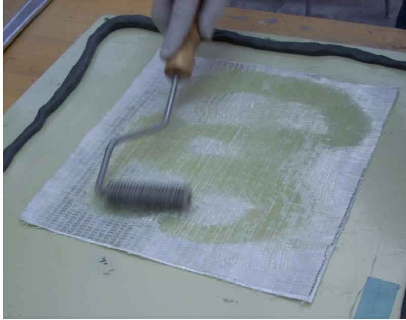
Fig 4.2-4: Manual Wetting of Fibers with a Hand Roller
