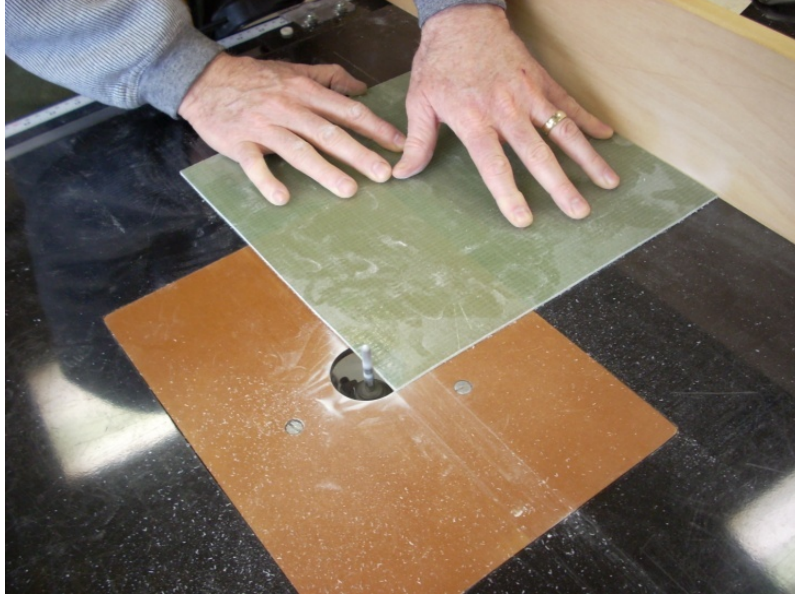
Fig 4.4-1: Panel Being Prepared with a Reference Edge
