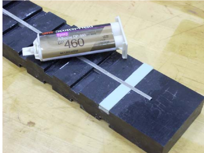
Fig 4.4-24: Overall Construction of ASTM D695M Compressive Specimens Bonded Together
