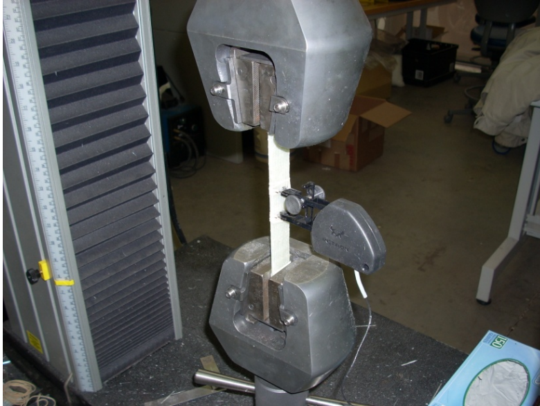
Fig 4.5-1: Tensile Test Setup, Extensometer Applied
