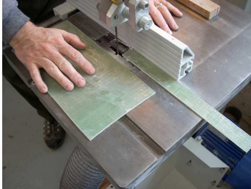
Fig 4.4-2: Tensile Strips Cut Using a Band Saw with a Guided Fence
