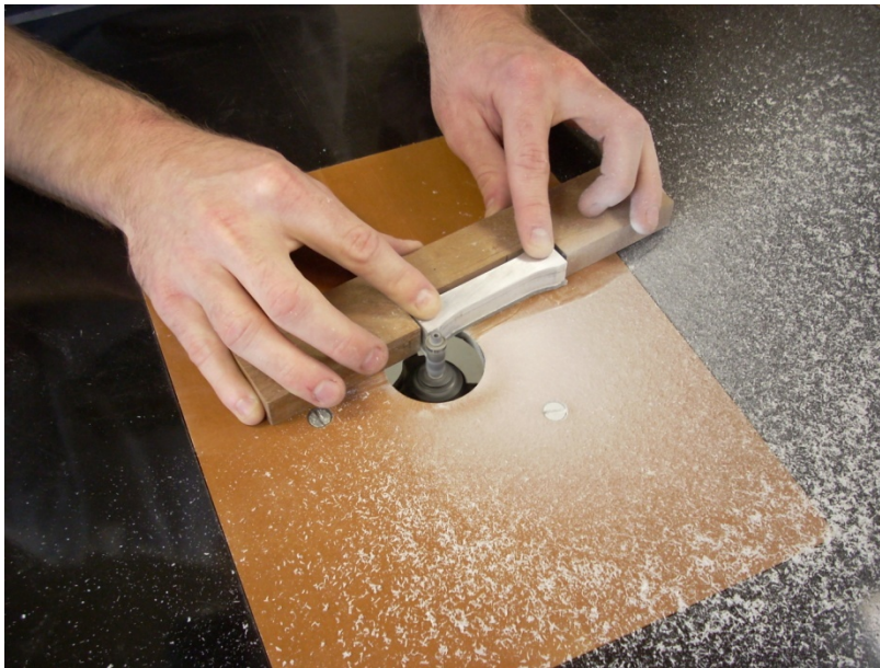
Fig 4.4-16: ASTM D695 Compressive Coupon Being Constructed with a Guided Router Bit
