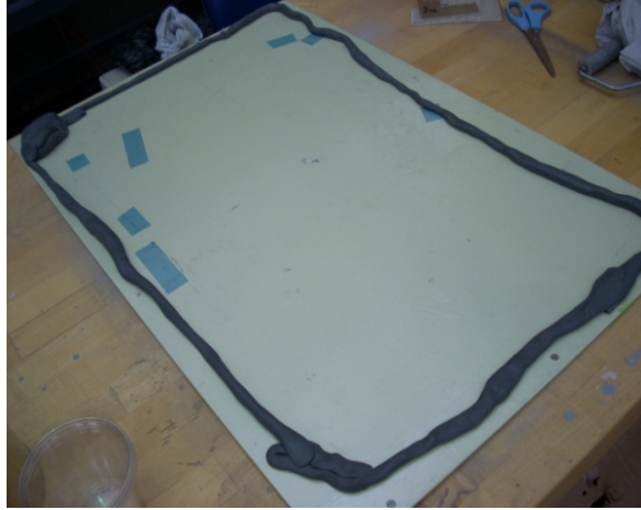
Fig 4.2-7: Covered Steel Plate with Duct Seal Lined Around the Perimeter
