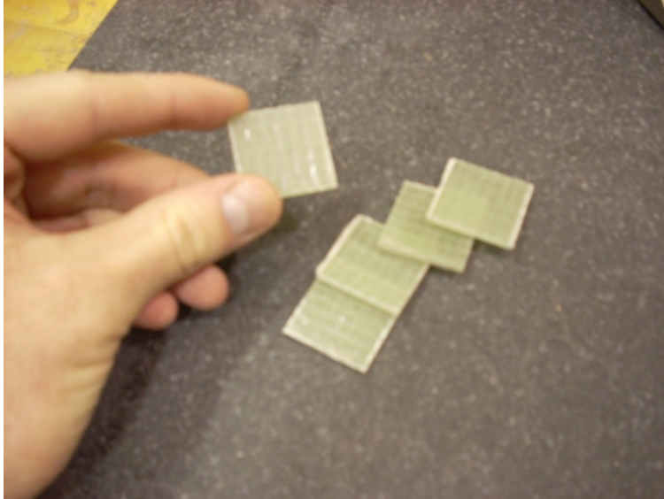
Fig 4.4-4: Finalized Ignition Loss Test Specimens, Dimensions of 1 inch by 1 inch
