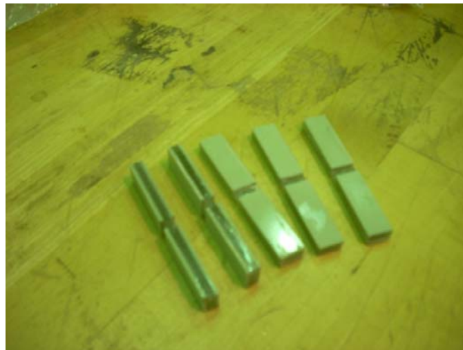
Fig 4.4-25: Finalized ASTM D695M Compressive Test Specimens
