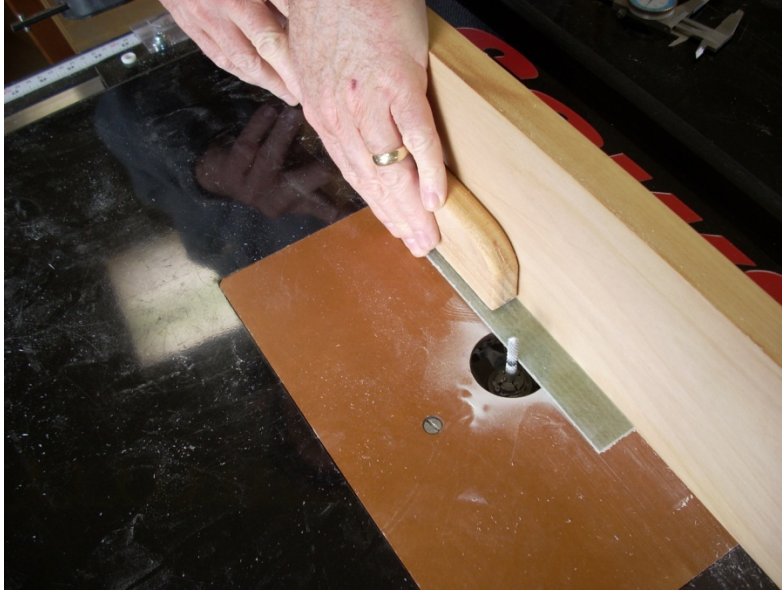
Fig 4.4-3: Tensile Coupon Edges Being Finished on a Router to a Width of 25.4 mm (1.0 in)
