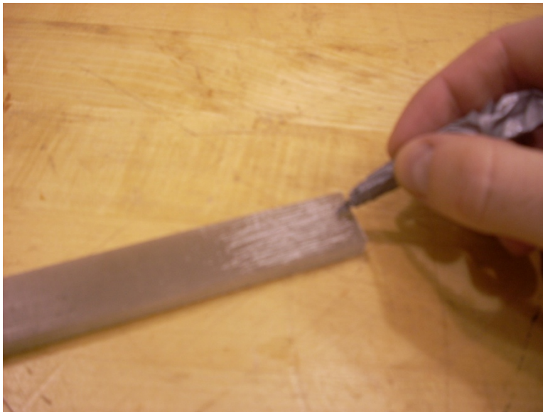
Fig 4.4-9: Tensile Specimen End After Surface Preparation for Adhesion
