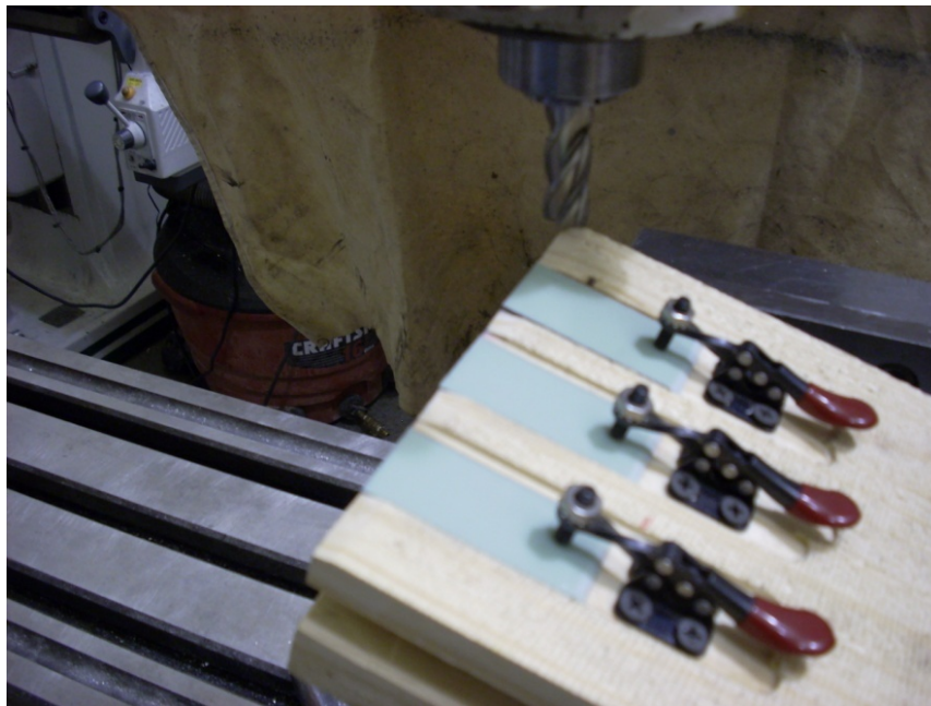
Fig 4.4-6: Tensile Tabs Held in Place by the Cutting Fixture
