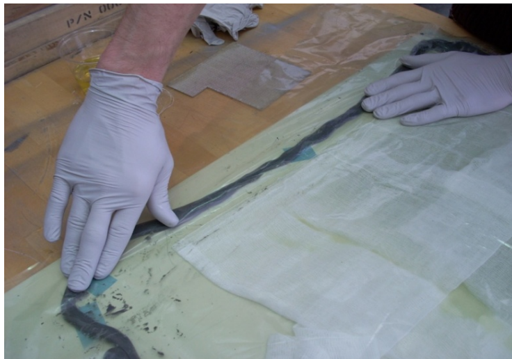
Fig 4.2-12: Final Layer of Anti-Bond Material Going Over Lay-Up
