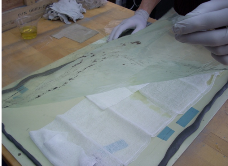
Fig 4.2-12: Final Layer of Anti-Bond Material Going Over Lay-Up
