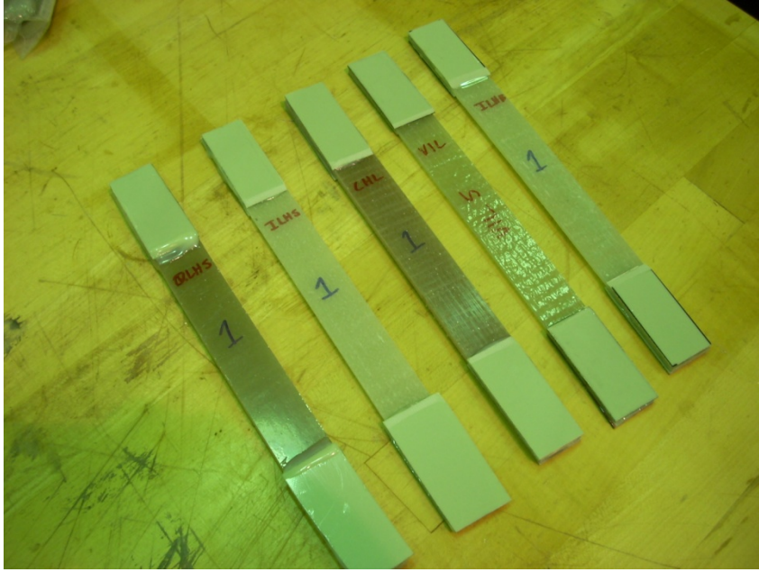
Fig 4.4-11: Finalized Tensile Coupons Bonded with Beveled Tabs
