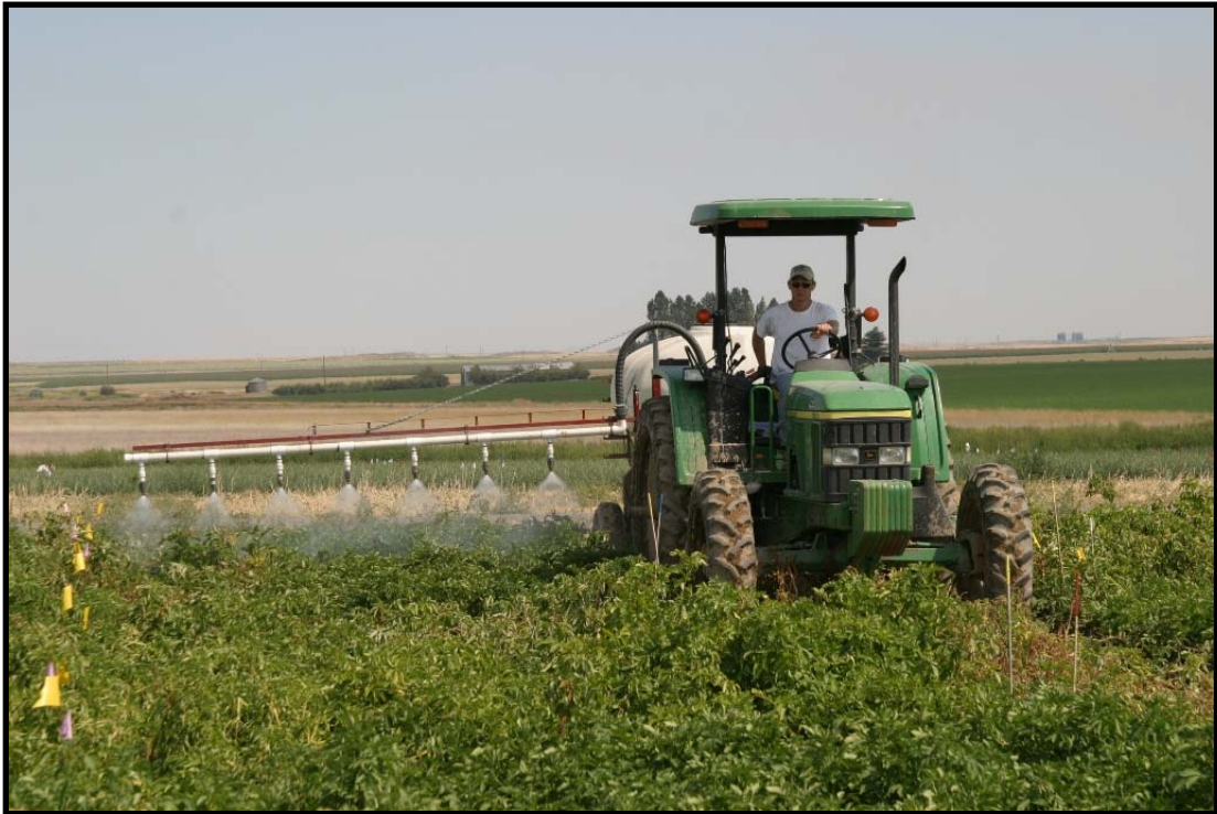
Fig. 1. Chemigation simulation unit applying in-season fertilizer treatments on the Othello Research station.
