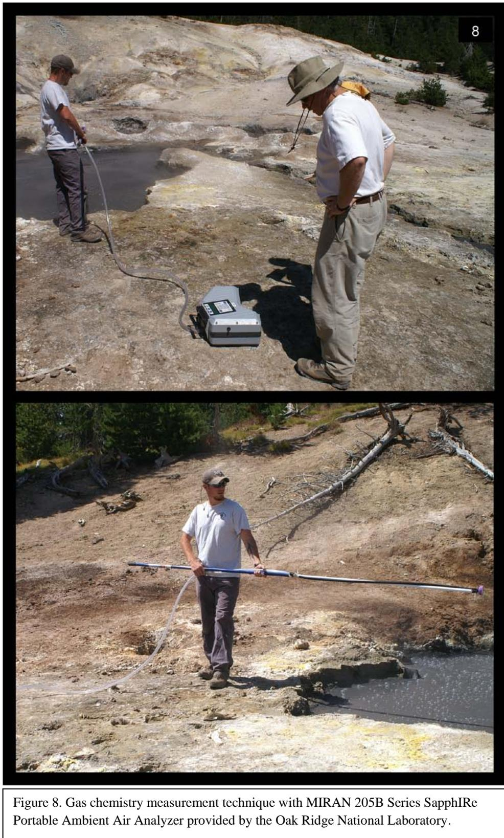
Figure 8. Gas chemistry measurement technique with MIRAN 205B Series SapphIRe Portable Ambient Air Analyzer provided by the Oak Ridge National Laboratory.
