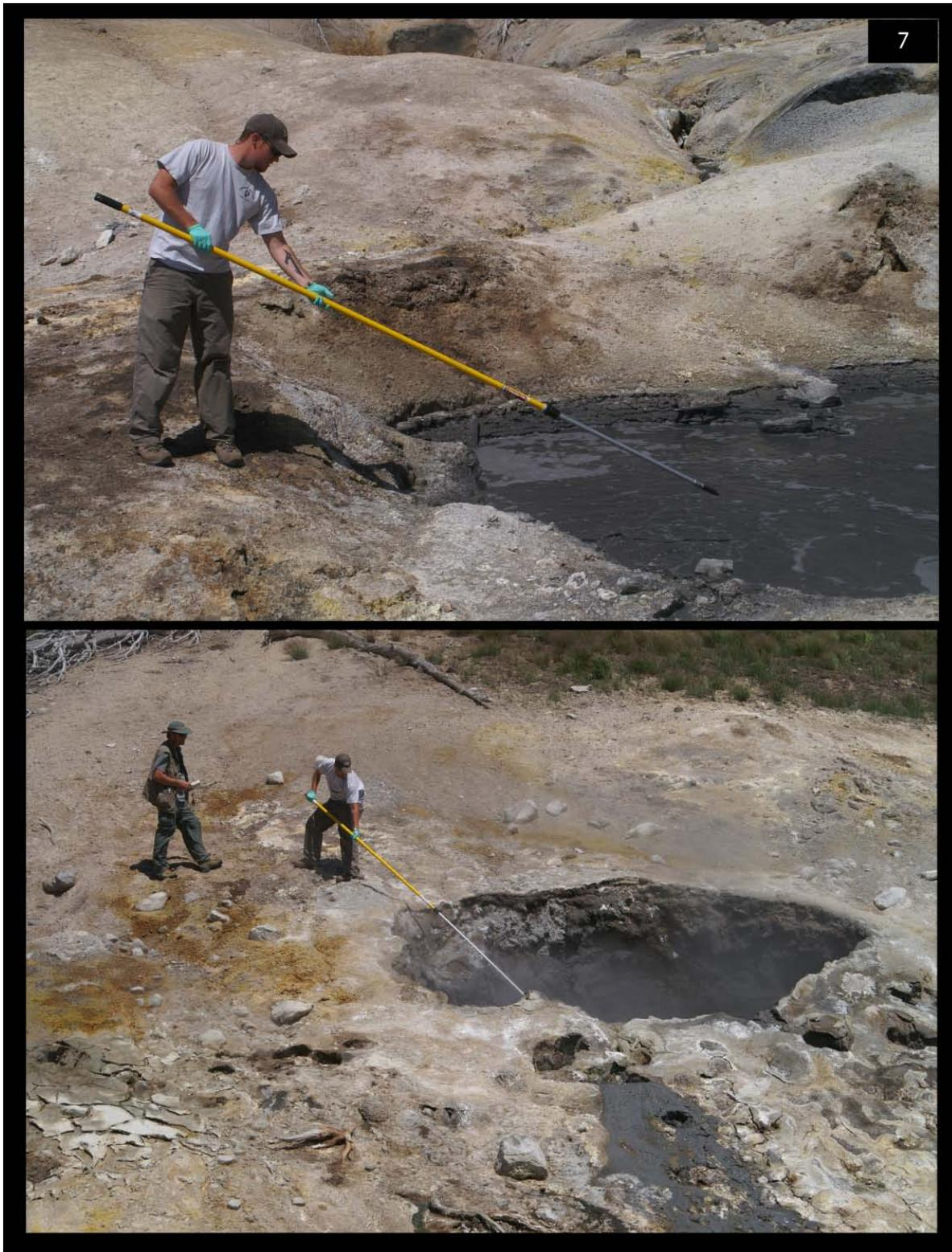
Figure 7. Sampling procedure using polyethylene bottle attached to an extendable aluminum pole.
