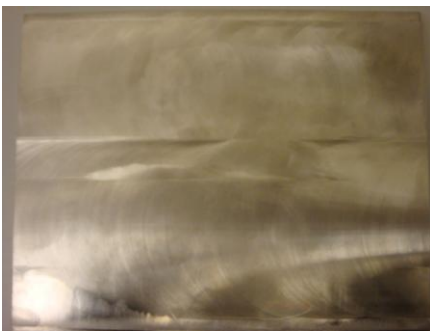
Figure 4.1.2-1: Titanium plate after alpha casing removal.
