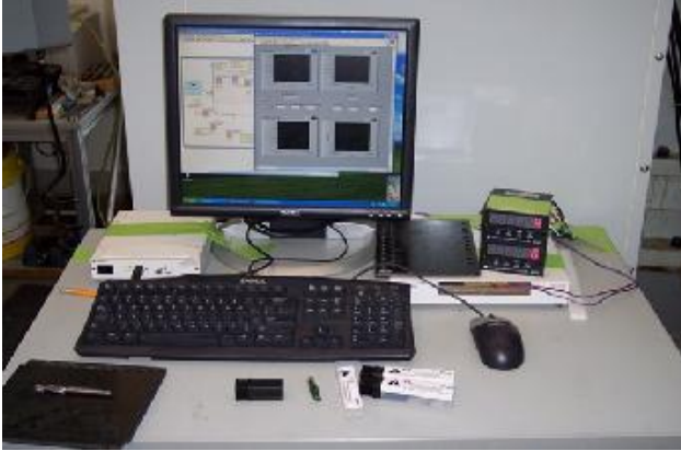
Figure 4.4.3-1: Thrust and torque signal capture setup.
