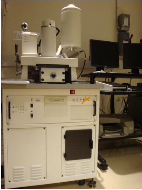
Figure 4.5.3-1: Scanning Electron Microscope (SEM) (Aspex Instruments).
