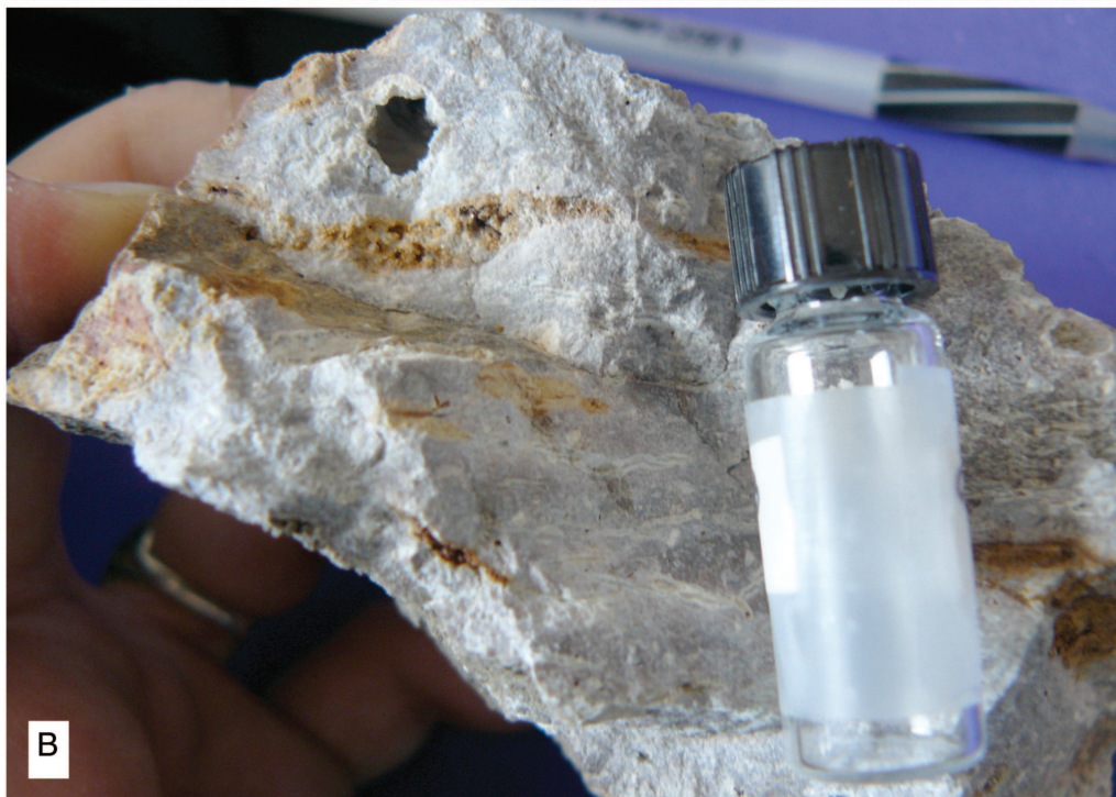
Figure 12. (A) Hand sample of accretionary lapilli tuff from Roberts Bay State Park. (B) Hand sample of capping rheomorphic densely welded tuff at Roberts Bay State Park showing recrystallized fiamme and lithophysal cavities. Note vial equals approximately 4 cm.
