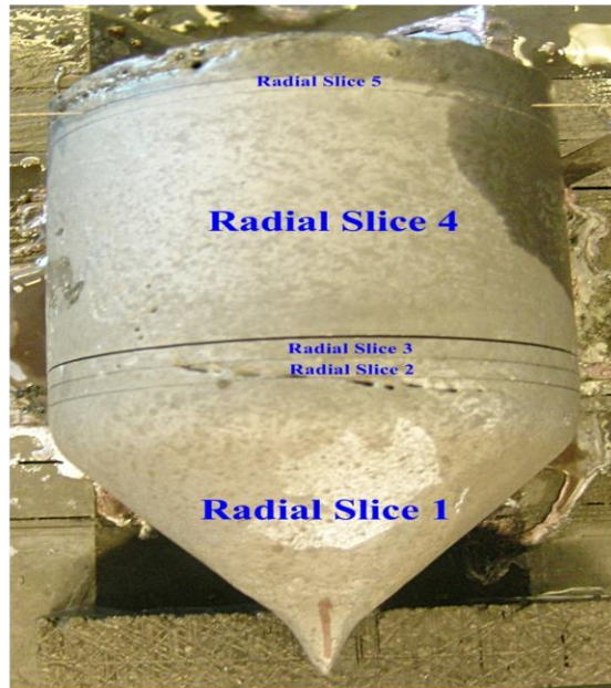
Figure 18(b): CG78(R2&R3) radial cut within the shoulder ~ (R2: Samples cut for MCA measurement and IR mapping; R3: General IR mapping)
