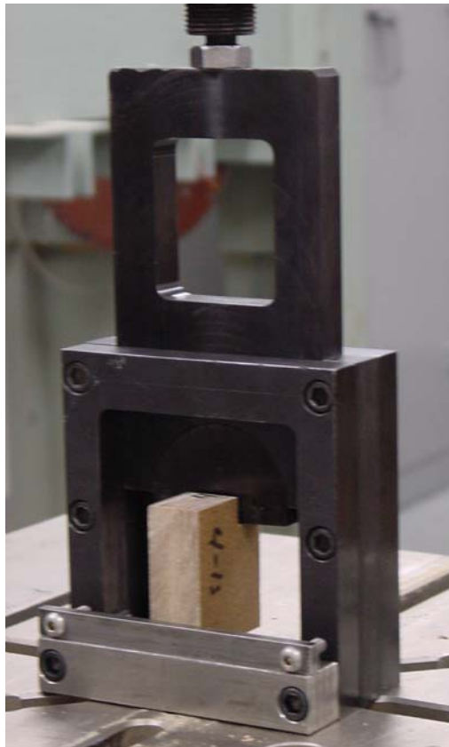
Fig. B Typical test setup for static shear block tests
