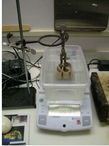
Figure A.1. Measurement setup on balance
