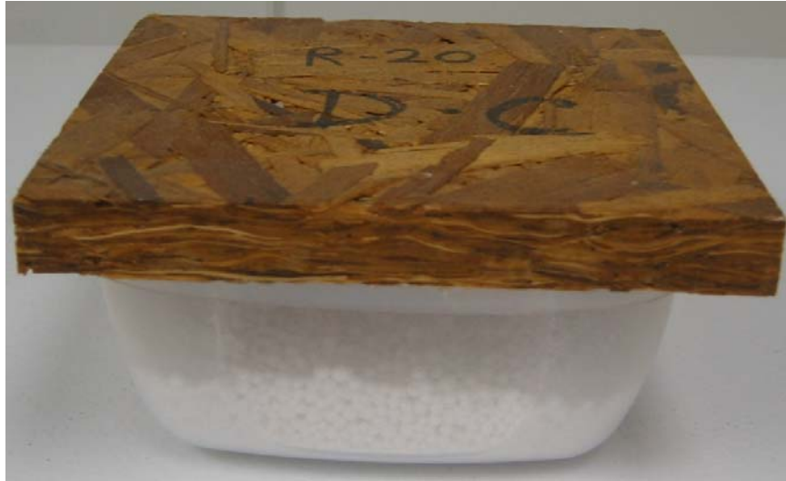
Figure 3.2 Test setup for water vapor transmission and permeance measurement.
