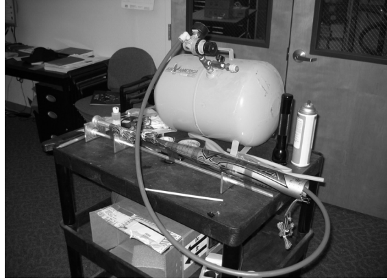
Figure 4.10 - Air tank and regulator used for application.
