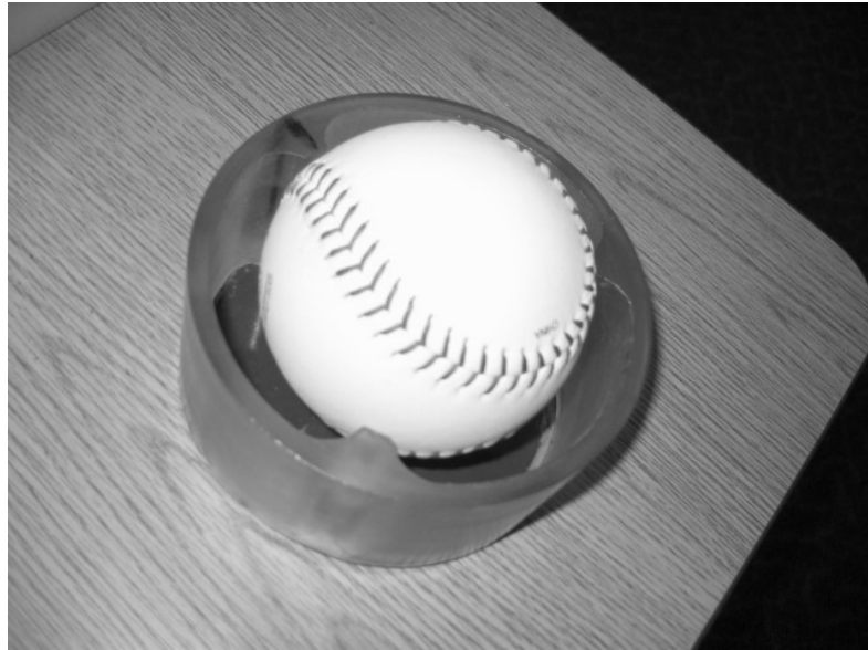
Figure 3.2 - Softball loaded in a sabot.
