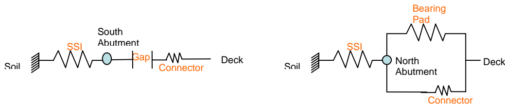
Figure 4.6.17: FE model of the soil, abutments, and deck interaction in the longitudinal direction
