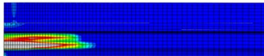
Figure 5-1: Maximum Principal Plastic Strain-Blast Above, Between Girders (Top View, Bottom View, Side View of Interior Girder)
