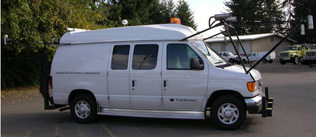
Figure A4.1 WSDOT pavement condition van.
