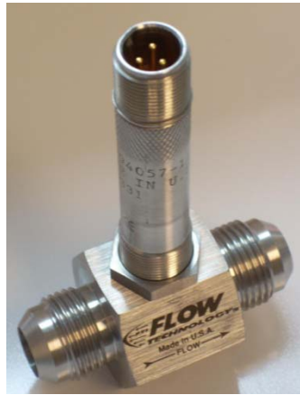
Figure 3.11 Flow meter to measure dynalene flow.
