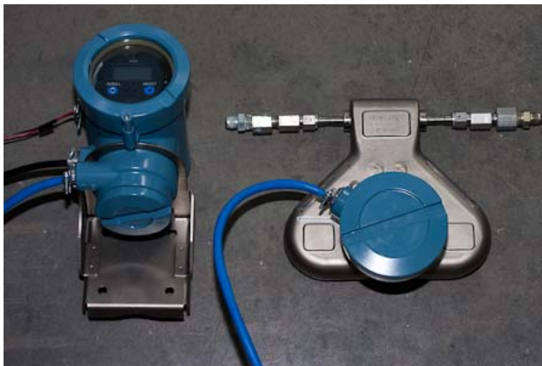
Figure 3.13 Coriolis flow meter with transmitter.
