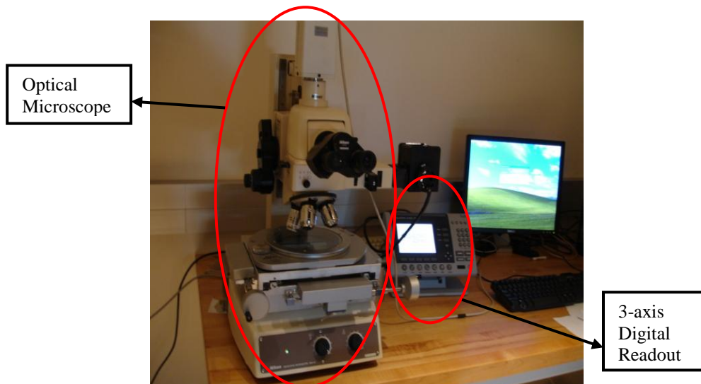
Figure 4.4.3-1. Measuring microscope (MM-40, Nikon, Japan) with 3-axis digital readout (Metronics, USA)
