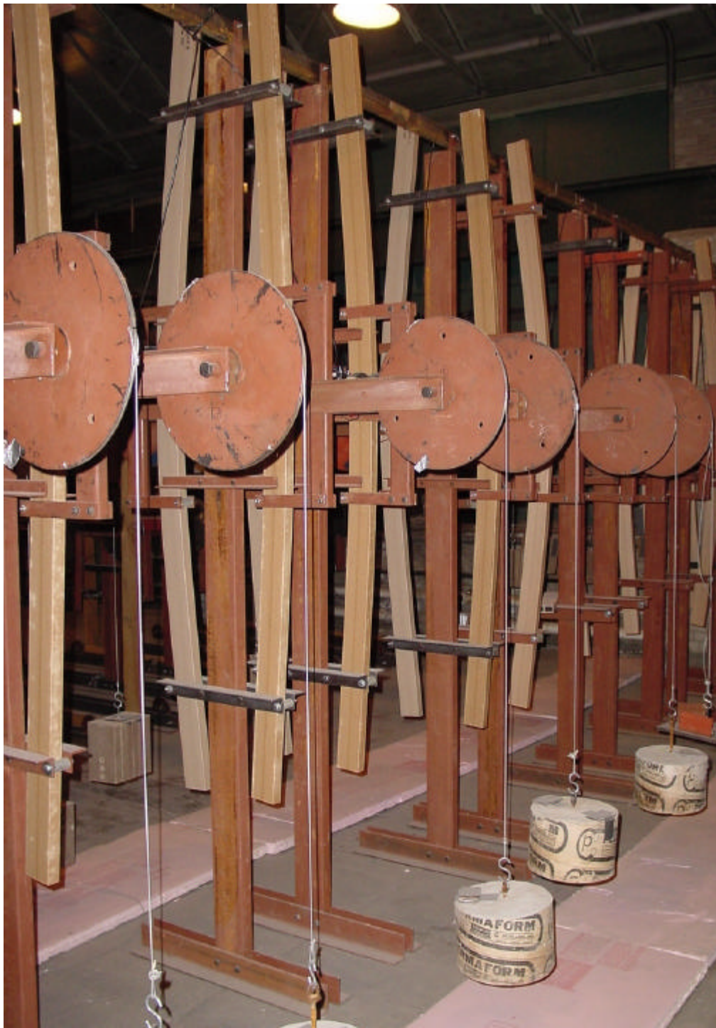
Figure 2-3: Load-Duration Test Frames
